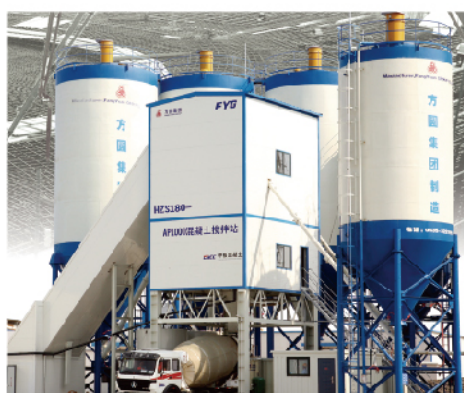
▲ 国内首台核电站建设专用混凝土搅拌站 The first domestic concrete batching plant for Nuclear power station
